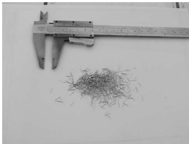
FIG. 1. Steel fibers used in the lightweight PC.
