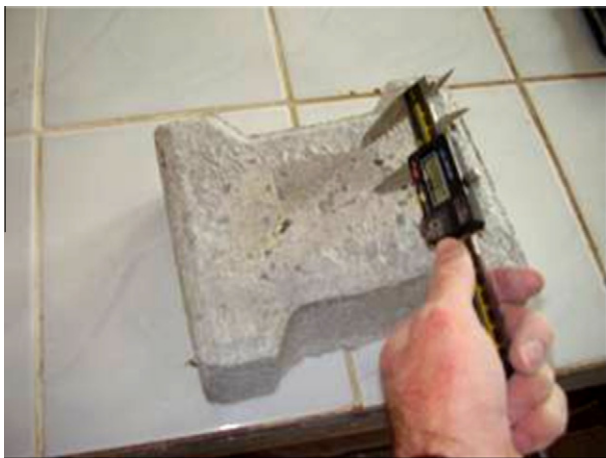
Fig. 4. Measuring of abrasion length of PCIB specimen.
